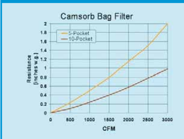
Camfil Farr's bag filters offer low pressure drop and are non-taxing to system airflow
