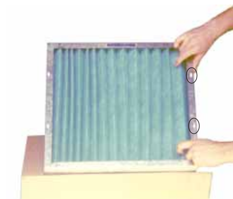
Spread the other side of the pleat out and tuck under the Pleat Retaining Notches, finally ensure Pleat is evenly spaced out in Frame.
